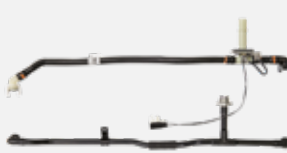
6 Battery Thermal Plastic Lines and Connectors
